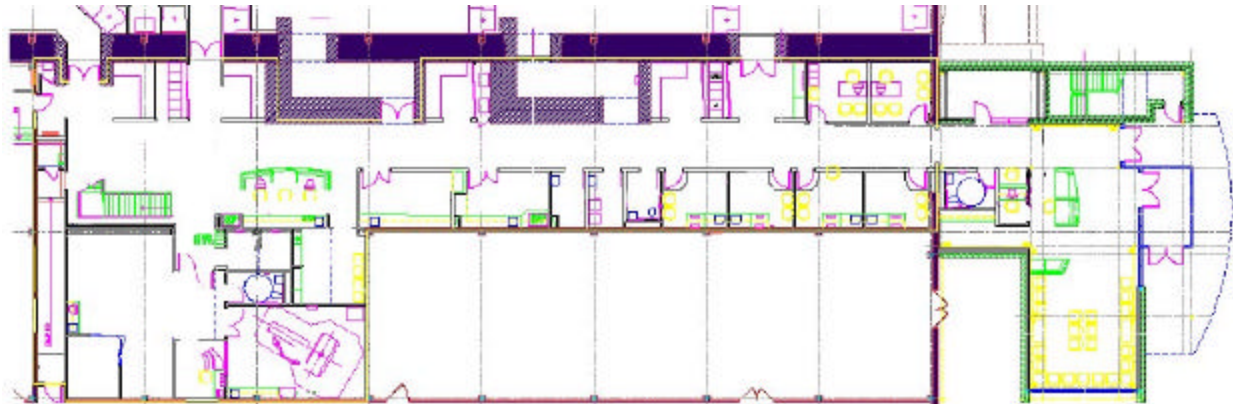
FIGURE 2. Clinic layout. The patient support facility has been constructed in the "low bay" of the IUCF building. The reception area at the far right is new construction. The CT/simulation suite and recovery areas are located at the lower left. RTT control consoles are located to the right of each of the maze entrances to the treatment rooms at the upper edge of the layout.
