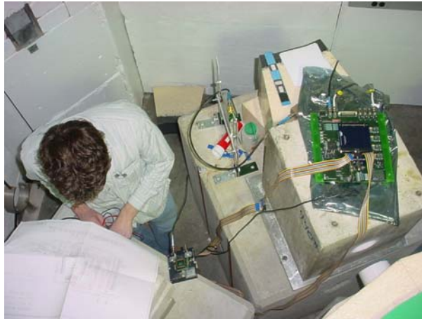
Figure 2: A microcircuit board is prepared for single event effect (SEE) testing at LENS.
