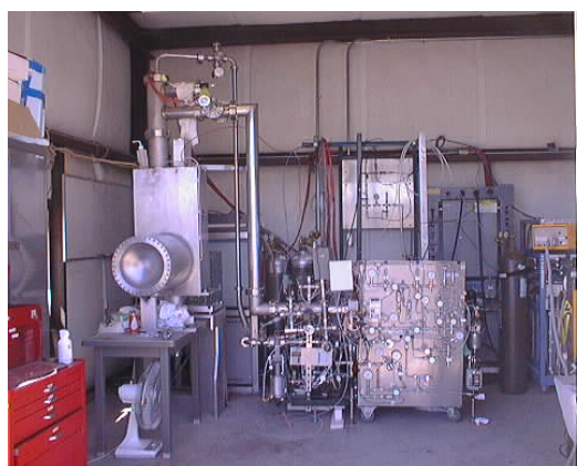
Figure 1: Liquid parahydrogen cryostat and gas handling system installed at Los Alamos in preparation for hydrogen tests.
