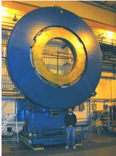
Fig. 2. Jim Sowinski standing in front of the STAR poletip. The detector built here will cover this full surface with many layers of lead and scintillator.
