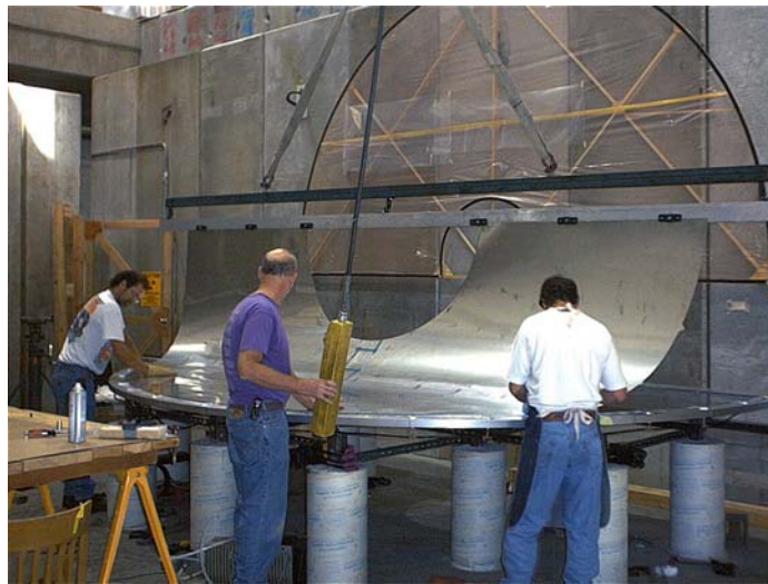
Fig. 4. Terry Sloan, Alan Eads and John Vanderwerp lowering the top layer of stainless steel onto a lamination.
