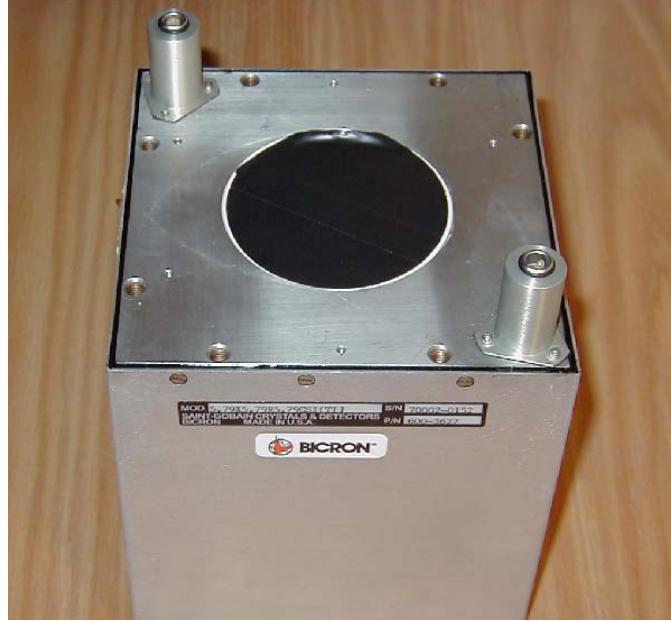
Fig. 6: Picture of one of the 48 CsI detectors for the NPDG experiment. The elements of the array are now at Los Alamos for final assembly.
