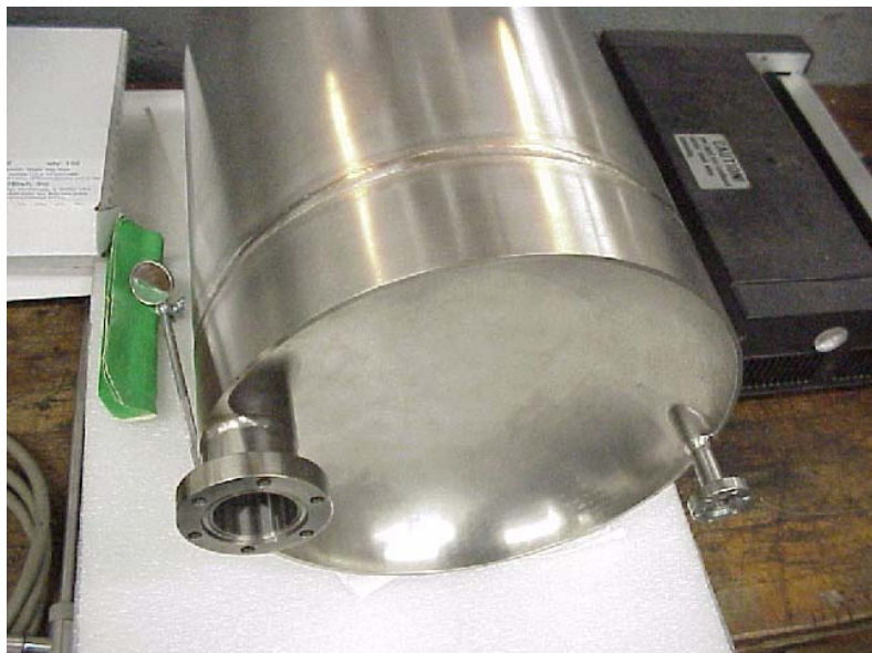
Fig. 7: Picture of the downstream portion of the titanium liquid hydrogen target vessel.
